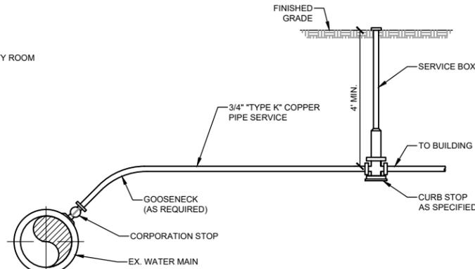
**TYPICAL WATER SERVICE INSTALLATION DETAIL**
